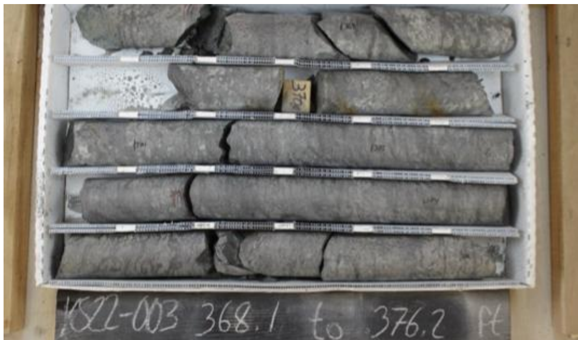
KS22-003 Core photo of magnetite rich ultramafic with nickel sulfide
